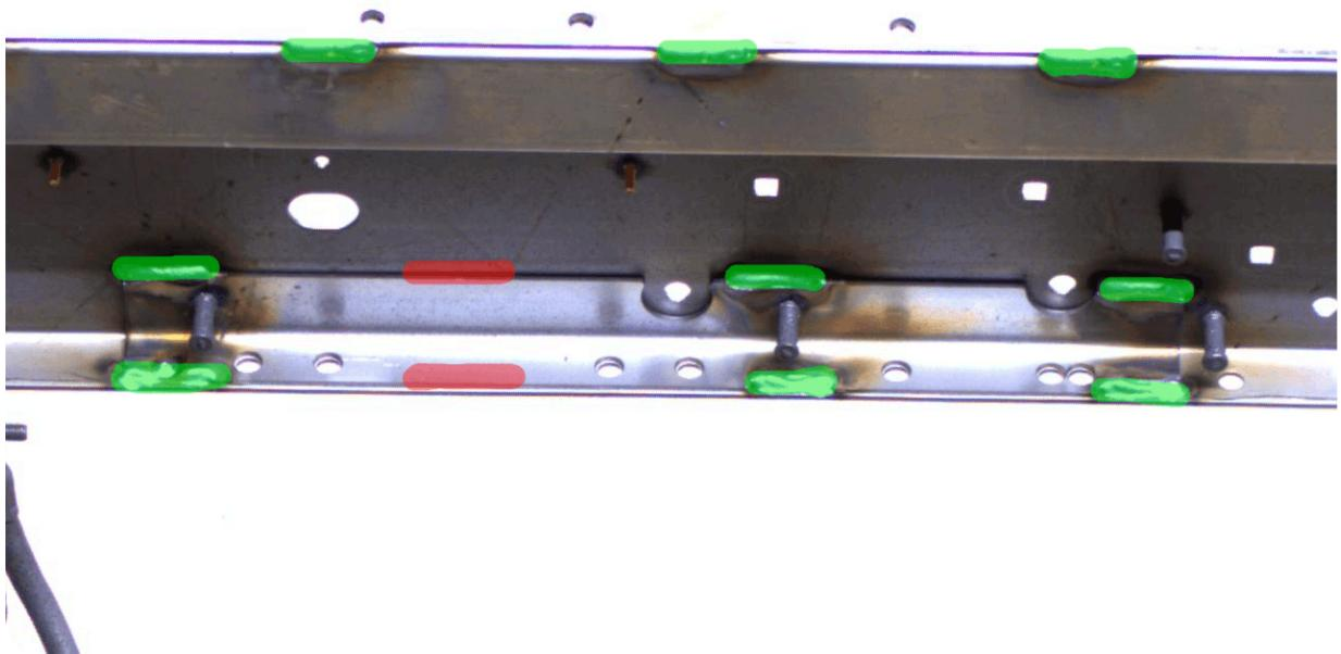
*Missing welds on input data marked in red → no match found with the CV algorithm*
